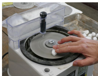
Fig. 2 A blade grinder for home use with a diamond disc
