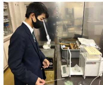
Fig.2 Heat the mixed powder using a microwave ovens
